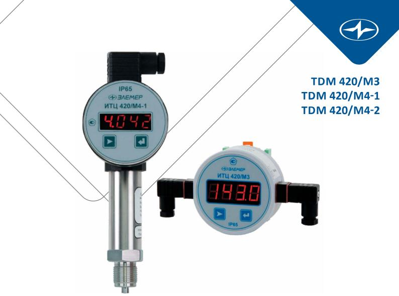
The Technological digital meters are connected to a 4...20 mA current loop and displays the current value. The scale is customizable. The TDM 420/M4-2 model has a built-in relay and can be used in process control and warning systems
