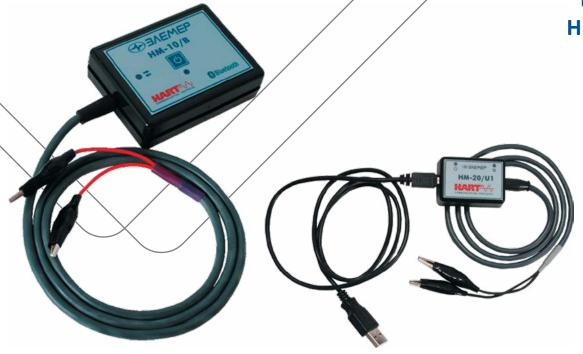
The HM-10/B and HM-10/U HART Modems connect a personal computer (PC) or a process control system with any HART-compatible smart devices (pressure, temperature, level, flow rate transducers)
