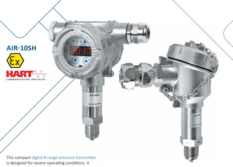
is designed for severe operating conditions. It continuously converts absolute pressure, manometric pressure, manometric negative pressure, differential pressure into a standard 4...20 mA current output with a HART output
