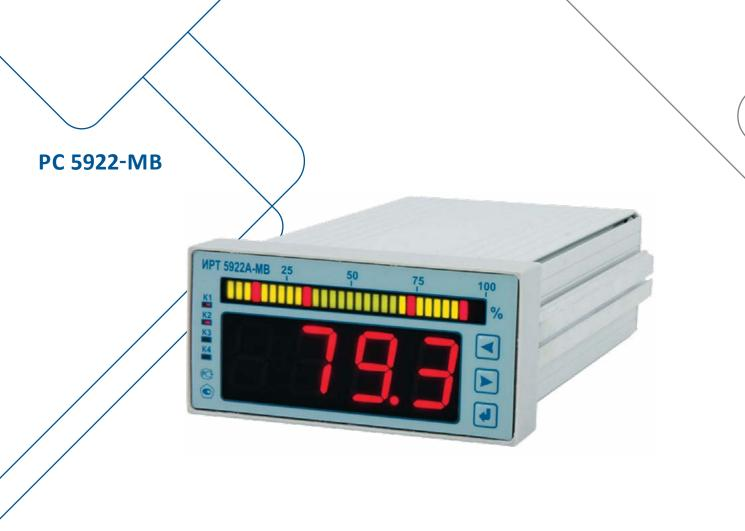
The PC 5922-MB Process Controllers measure and control temperature and other non-electric values converted into DC current or Power signals and DC active resistance. The PC can be integrated into Modbus RTU-based systems with the built-in interface module
